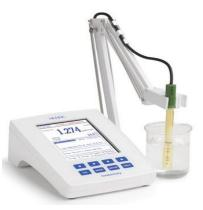
The HI5321 is feature-rich with 4-point calibration, auto-sort, data logging, alarm settings, comprehensive GLP and more, while maintaining ease of use with a dedicated key for simple operation and virtual keys that guide the user through configuration options [6]. Capacitive touch pad HI5321 pre-programmed with USP
